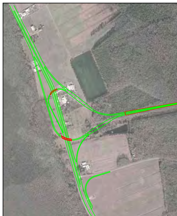
Compressed Y Interchange Design NCTA Selected Concept
